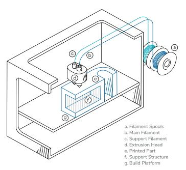
One of the most common forms of material extrusion is Fused Deposition Modeling (FDM), and perhaps the bestknown additive manufacturing process. FDM extrudes a thermoplastic filament through a heated nozzle and onto a build platform. The material then solidifies as it cools, although not until it fuses to adjacent layers. FDM uses a wide variety of thermoplastic filaments, including ABS, PLA, nylon, PC, ULTEM, and more complex filaments (metal and wood).
