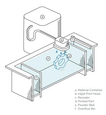
The Binder Jetting Process is similar to material jetting, but uses powdered material and a binding agent. Nozzles deposit tiny droplets of a binder on an ultrafine layer of a broad range of powdered materials (metal, ceramic, glass, etc.). Multiple layers result from the powder bed moving downward after each layer is created.
