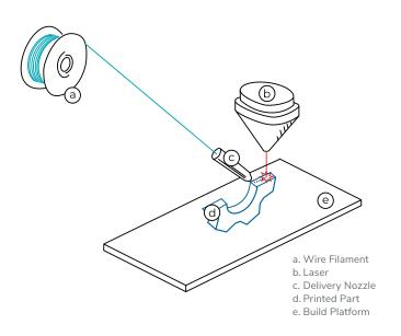
Directed Energy Deposition (DED) uses highly focused thermal energy (laser, electron beam, or plasma arc) to melt and fuse material jetted into the heated chamber from either powdered metal or wire filament. DED closely resembles welding and is commonly used to repair and maintain existing parts, although it can be used to deposit material directly onto a build tray.
