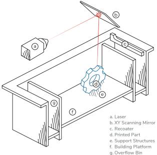
As the name suggests, Powder Bed Fusion (PBF) involves melting particles to fuse them together. Particles of plastic or metal powder are either "sintered" (partially melted) or fully melted using thermal energy in the form of a laser, beams of electrons, or a heated print head.
