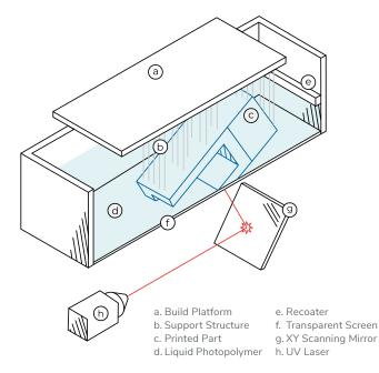
Vat photopolymerization uses liquid rather than powder or filament. Printing techniques vary, but they all use photopolymer resins – often tough, transparent and castable materials. The resins are cured using UV light directed across the surface of the resin.
